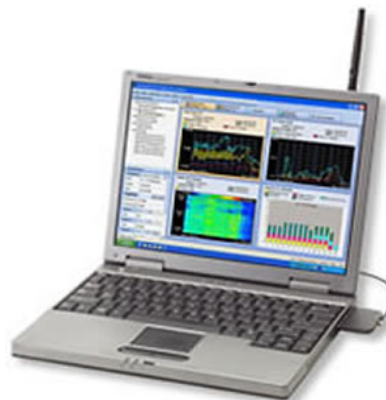
Laptop running AirMagnet WIFI Analyzer
