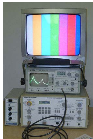
Alignment and testing using a video signal generator and Spectrum analyzer
