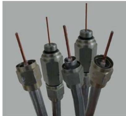
Hardline Coax cable
