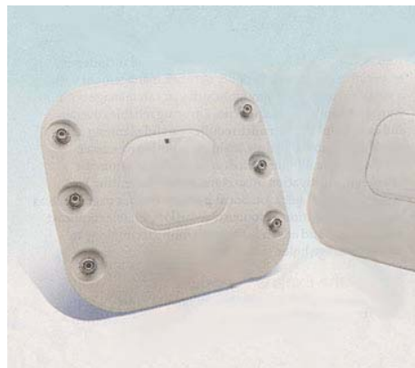
802.11N access point with Multiple Input Multiple Output antennas
